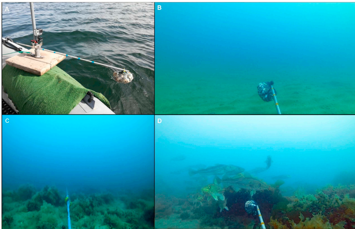
Fig. 2. Multi-pane overview of the RUVS used for monitoring in this study. A) BRUVS setup with a bait arm extended within the FOV, marked with tape at 10 cm increments used for visibility estimates, B) Sand site with low cobble coverage recorded by a BRUVS, C) Reef site with high cobble coverage, recorded by an UBRUVS with a sponge attached to a rope at 1 m distance from the camera for visibility estimates and D) a school of Atlantic cod ( Gadus morhua ) passing the FOV, recorded at intermediate cobble coverage by a BRUVS at one of the reef sites.
