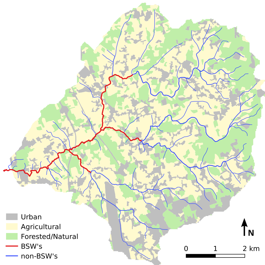
Fig. 8. The Water Framework Directive's measures apply only to Bodies of Surface Water (BSW). However, non-BSW may correspond to a large part of the hydrographic net, draining water from lands impacted by human activities. Restoration efforts targeted only at BSW may be ineffective if stressors exist further upstream, on non-BSW. The river Onda (Portugal) is shown as an example. Notice that non-BSW cross through areas used for agriculture and urbanisation.
